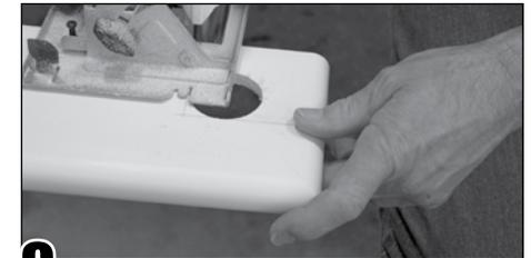
**9** Cut along the depth and width markings. Do not cut past the circle you drilled. Continue with step 8 of the Basic Installation Instructions.
