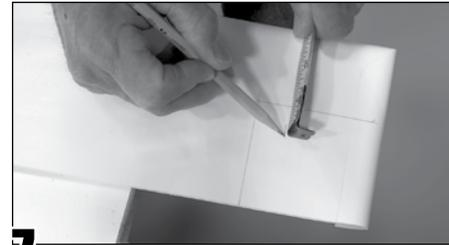
**7** Extend the width and depths markings you made in steps 5&6. Mark the radius measurement as shown in the diagram below.
